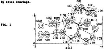
A least-squares refinement of the 2670 independent data resulted in an R-factor of 11.8%. The average C-C bond distance is 1.55A and the average C-N bond distance is 1.51A with standard deviations of at most .023A for the individual bond lengths.
